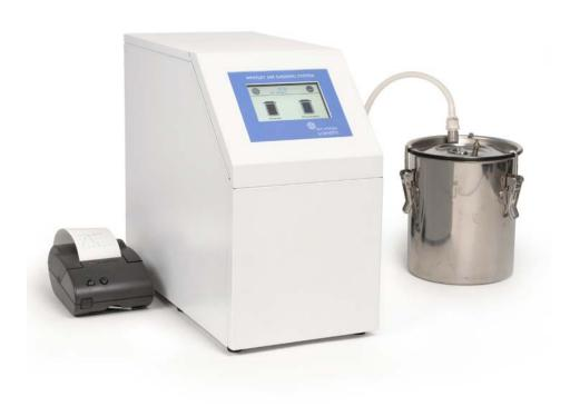
The Whitley Jar Gassing System is the most convenient, rapid and costeffective way to achieve either anaerobic or microaerobic conditions within a gas jar – under two minutes to create an anaerobic environment and just 15 seconds to achieve microaerophilic conditions.\*
