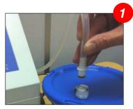
Simply attach the connector from the Whitley Jar Gassing System to the jar containing your samples. Remember to include a catalyst sachet in the jar when preparing anaerobic conditions.
