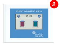
The Whitley Jar Gassing System uses separate cycles to prepare anaerobic or microaerophilic conditions.
